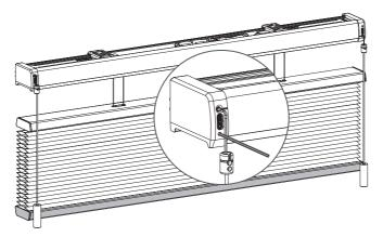
Pair the bottom rail motor to an empty channel on the remote. (see step 1)
