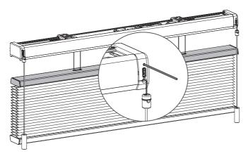
Pair the middle rail motor to an empty channel on the remote. (see step 1)
