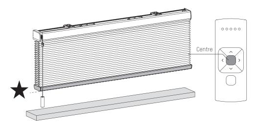
**Deactivate program mode**Shortly press the program button to deactivate program mode. The blind stops stepping and can be operated.
